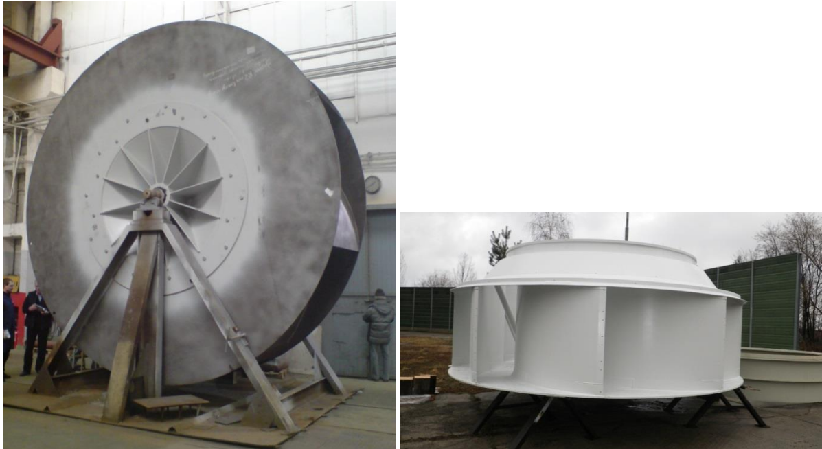
Fig. 3b.1. New rotating unit of the centrifugal fan WPK-5.35 on testing bench and ready for installation
